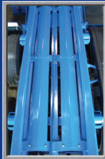
Simple Reeving Cylinder Cover Replacement
